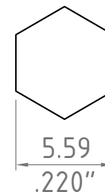
Recommended Crimping Dimensions for Ferrule
